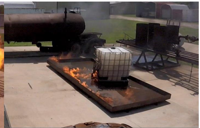
Figure 3.6: Pool fires and burning IBC following flare-up
