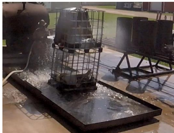
Figure 3.12: After extensive fire-fighting, IBCs are extinguished
