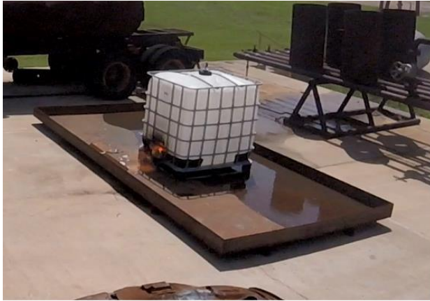
Figure 3.3: IBC inflation and initial vapor release
