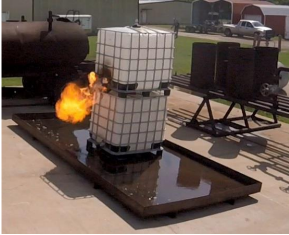
Figure 3.8: Tote inflation and initial vapor release
