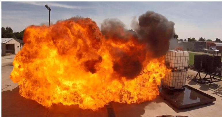
Figure 3.10: Ignited vapors create fire ball extending nearly 40 feet
