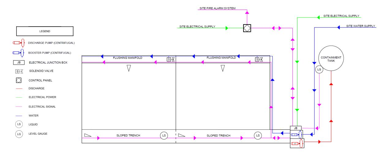
ONLY 2 ZONES SHOWN FOR REFERENCE. LARGE AIRCRAFT REQUIRE ADDITIONAL SECTIONS, FLUSHING MANIFOLDS, AND TRENCHES.
