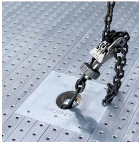
Figure 8-4: ILDFA tie down point example with aircraft chain connection
