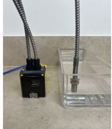
Figure 14-1: Liquid detection sensor components and operations
