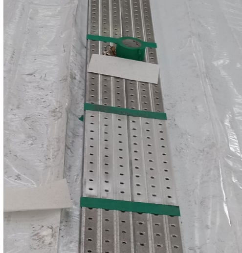
Figure 2.7 : Area of Safespill floor taped off and prepared for dry testing
