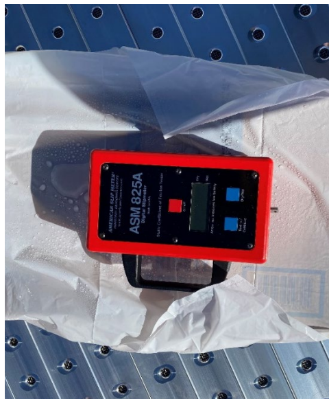
Figure 2.8: Sensors of ASM 825A allowed to sit in standing water for 5 minutes to absorb moisture
