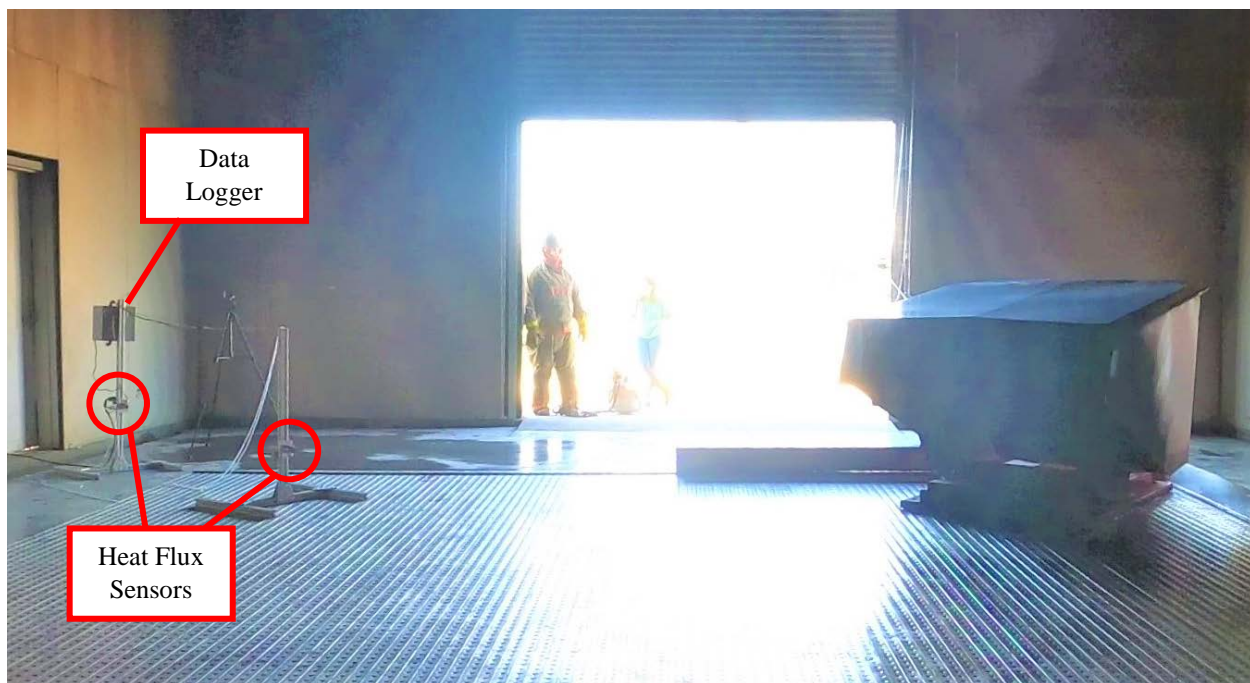
Figure 2-4: Test layout shown from trench side of floor. Heat flux sensors mounted to stands on left side of frame.
