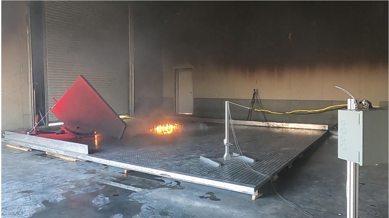
1:20 – Area of fire is reduced to approximately 0.8 m 2 (9 ft 2 ). Heat flux is undetectable to both sensors at this point.
