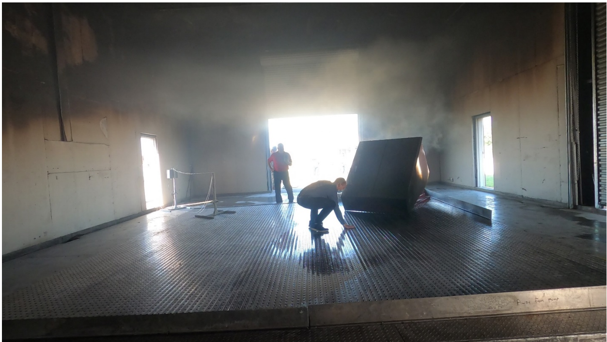
2:33 – Fire is extinguished without intervention, supervising fire fighter gives “all clear” and the floor is cool to touch.
