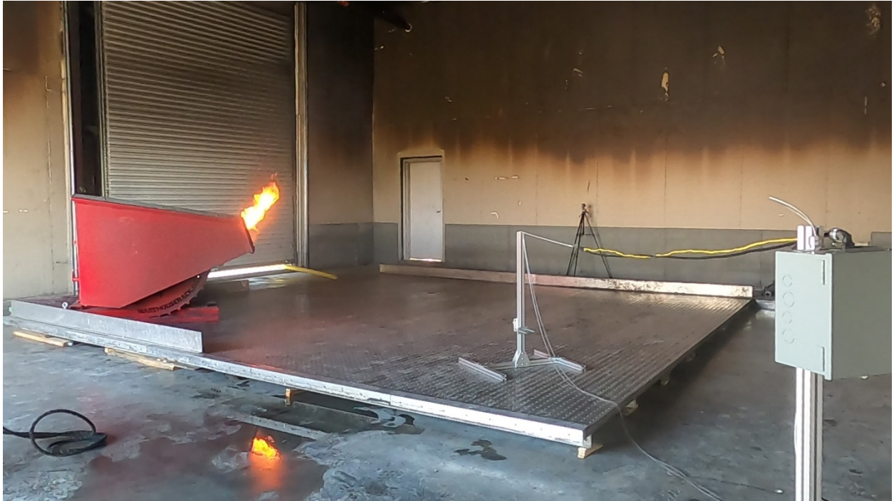
Preburn - Fuel is ignited using propane torch and allowed to burn inside enclosed hopper for 5 seconds before dump begins.
