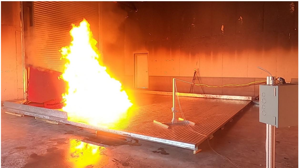
Spill initiated - As hopper begins to dump, fuel flows onto floor creating a large flare-up.
