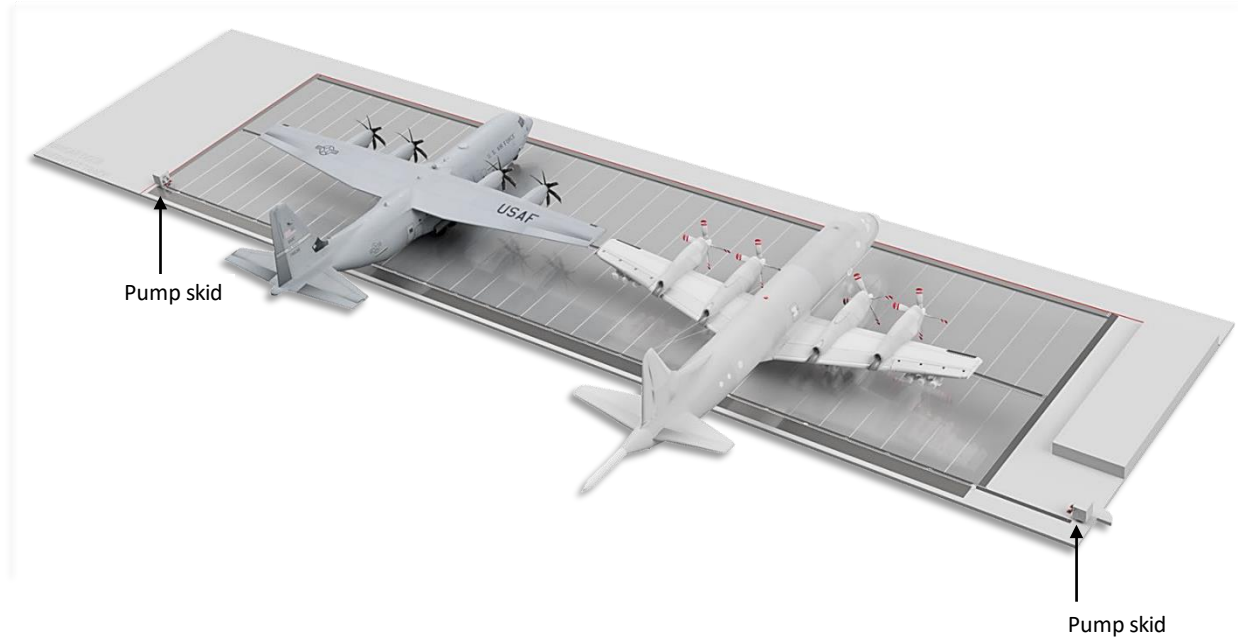
Figure 10-2: Render of ILDFA Layout with pump skids on opposite sides of the system
