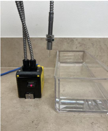
Figure 12-1: Liquid detection sensor components and operations
