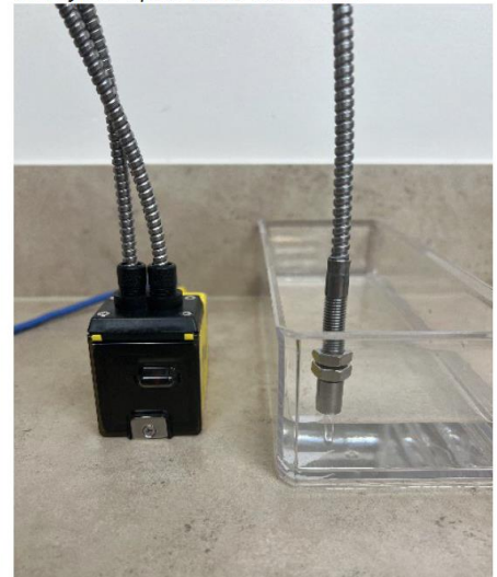
Figure 12-1: Liquid detection sensor components and operations
