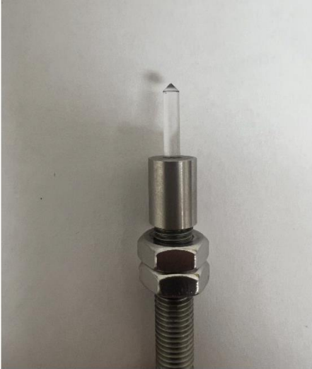
Glass Prism at end of fiber optic cable
